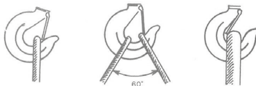
"IMPROPER" SLINGING CASES
